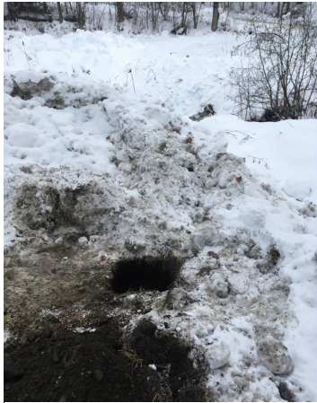
Figure C30. A hand auger and shovel were used to assess soil conditions and infiltration potential.
