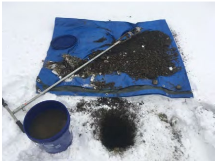
Figure C20. A hand auger and shovel were used to assess soil conditions and infiltration potential.
