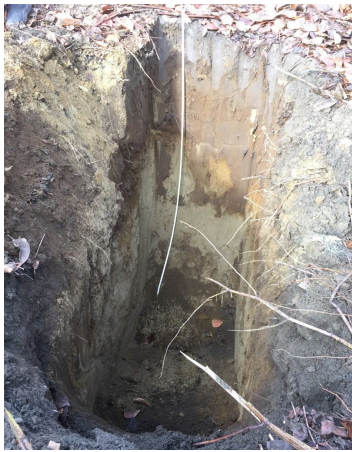
Figure A21. An excavator was used to assess soil conditions and infiltration potential.
