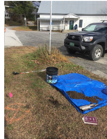
Figure A16. Soils were assessed in the greenspace adjacent to the Post Office where the proposed infiltration practice would be located.
