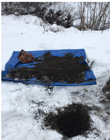
Figure C26. A hand auger and shovel were used to assess soil conditions and infiltration potential.
