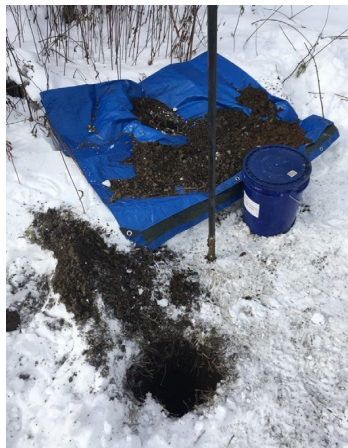
Figure C17. A hand auger and shovel were used to assess soil conditions and infiltration potential.
